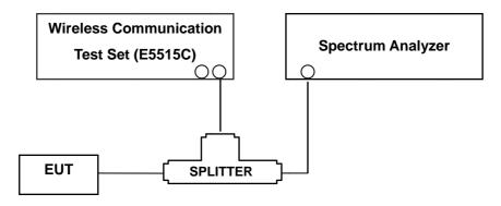
(Configuration of conducted Emission measurement)
