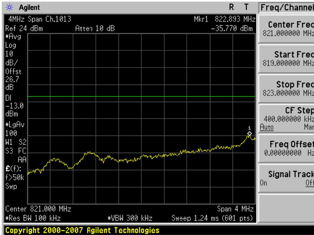
■ CDMA EVDO\_Rev.0 MODE (1013 CH.) 4 MHz Span
