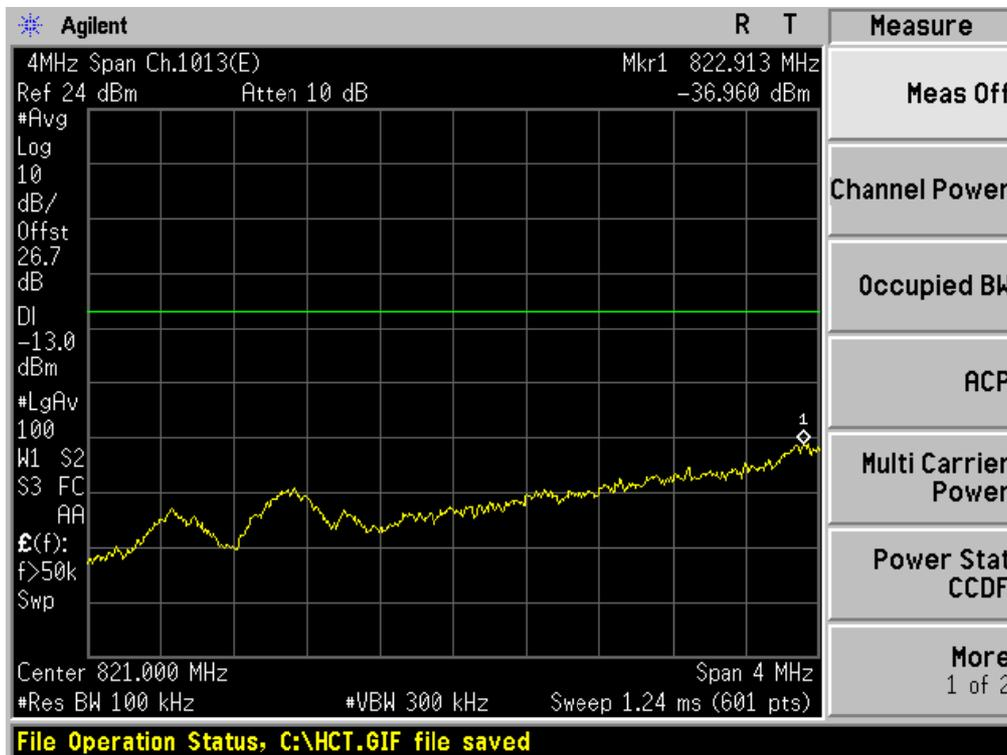
■ CDMA EVDO\_Rev.A MODE (1013 CH.) 4 MHz Span
