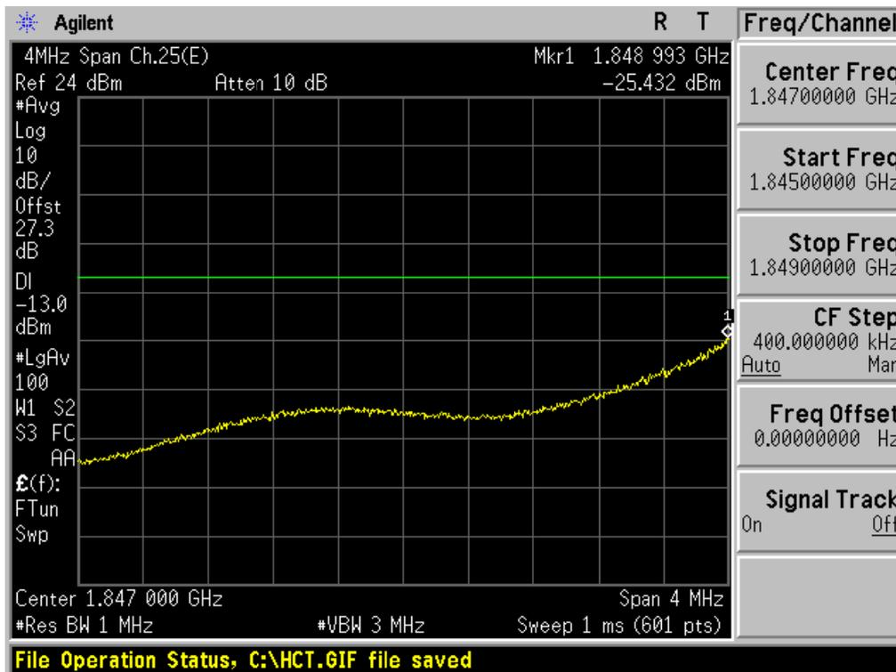
■ PCS EVDO\_Rev.A MODE (25 CH.) 4 MHz Span
