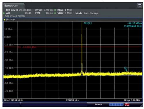
■ PCS MODE (600 CH.) 3.3 GHz ~ 10 GHz Conducted Spurious Emissions - 2
