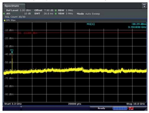
■ PCS MODE (25 CH.) 10 GHz ~ 20 GHz Conducted Spurious Emissions - 3
