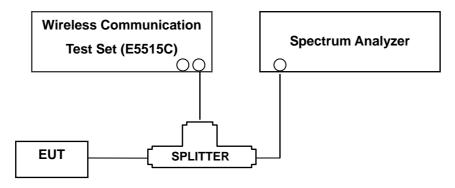
(Configuration of conducted Emission measurement)
