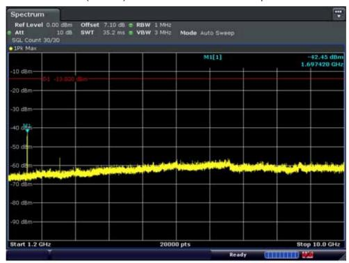
■ PCS MODE (25 CH.) 30 MHz ~ 3.3 GHz Conducted Spurious Emissions - 1
