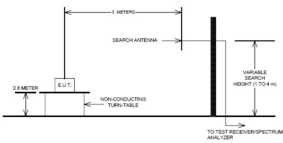
The measurement facilities used for this test have been documented in previous filings with the commission pursuant to section § 2.948. The open field test site is situated in open field with ground screen whose site attenuation characteristics meet ANSI C63.4 –2003. A mast capable of lifting the receiving antenna from a height of one to four meters is used together with a rotatable wooden platform mounted at three from the antenna mast.
