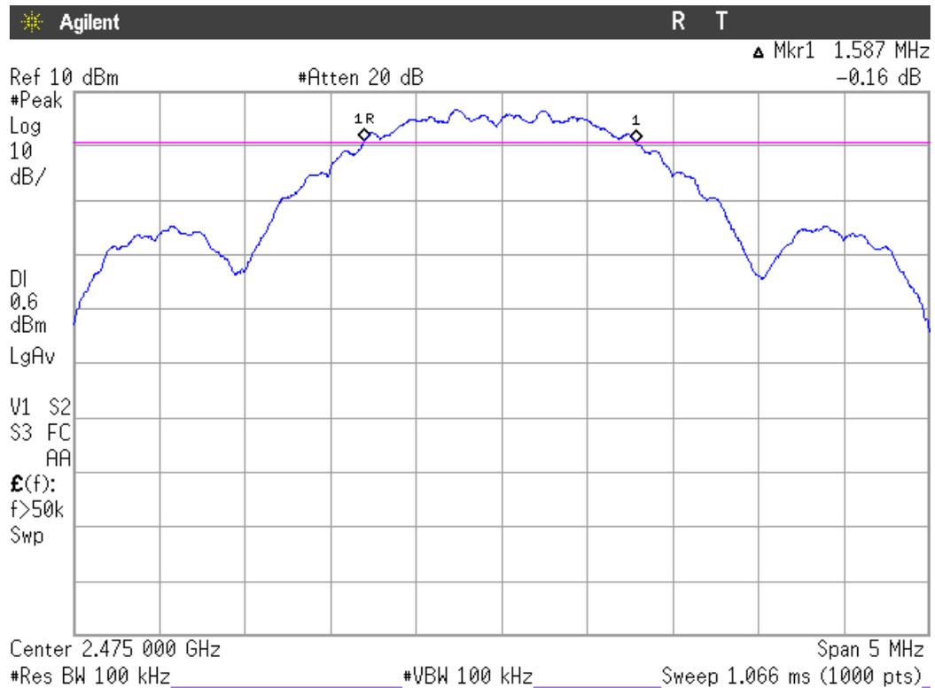
**Section 15.247 Subclause (b). Maximum output power and antenna gain / RSS-210 A8.4.
