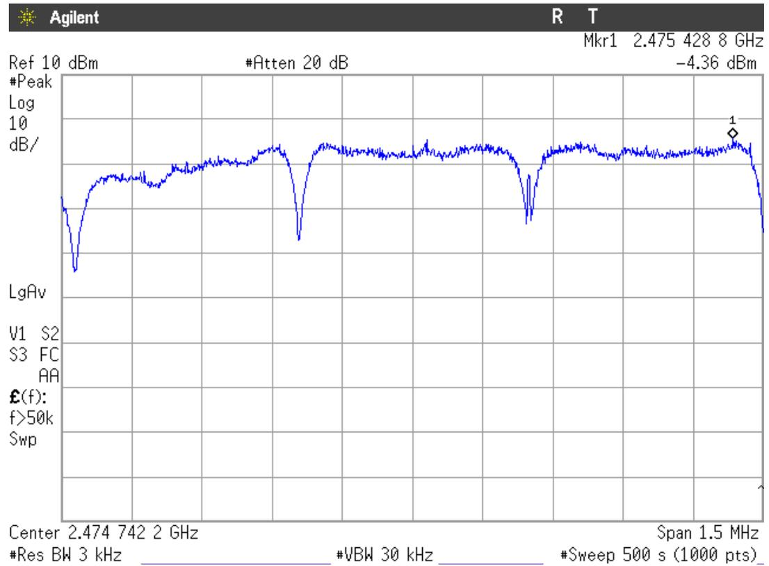
**Section 15.247 Subclause (d). Emission limitations radiated (Transmitter) / RSS-210 A8.5.**
