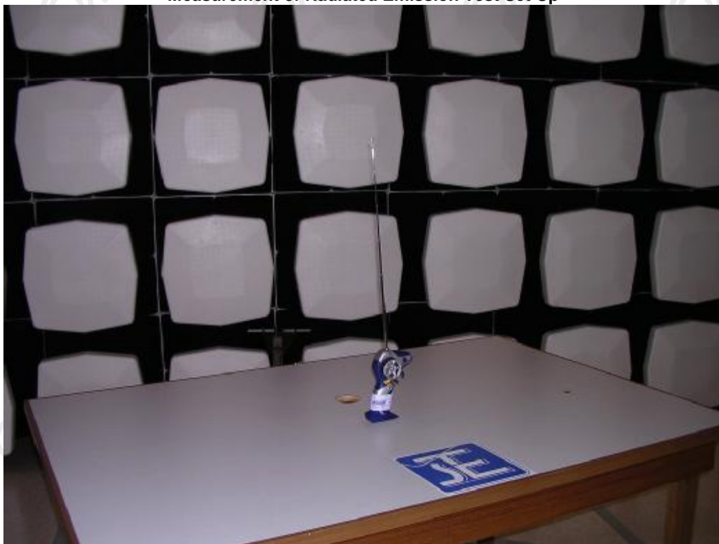
Measurement of Radiated Emission Test Set Up
