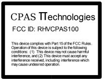
The label is approximately 2.25 by 1.75 inches. It will be centered on the metal RF shield of the SS100.
