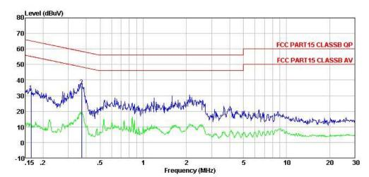
: FCC PART15 CLASSB QP LISN-2012 LINE : DryBuddyFLEX receiver Condition EUT
