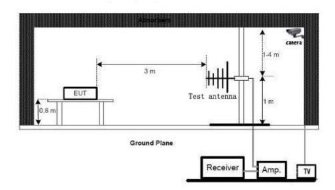
The EUT is located in a 3m Semi-Anechoic Chamber, the antenna factors, cable loss and so on of the site as factors are calculated to correct the reading.
