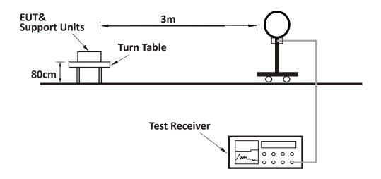
For Radiated emission 30MHz to 1GHz:
