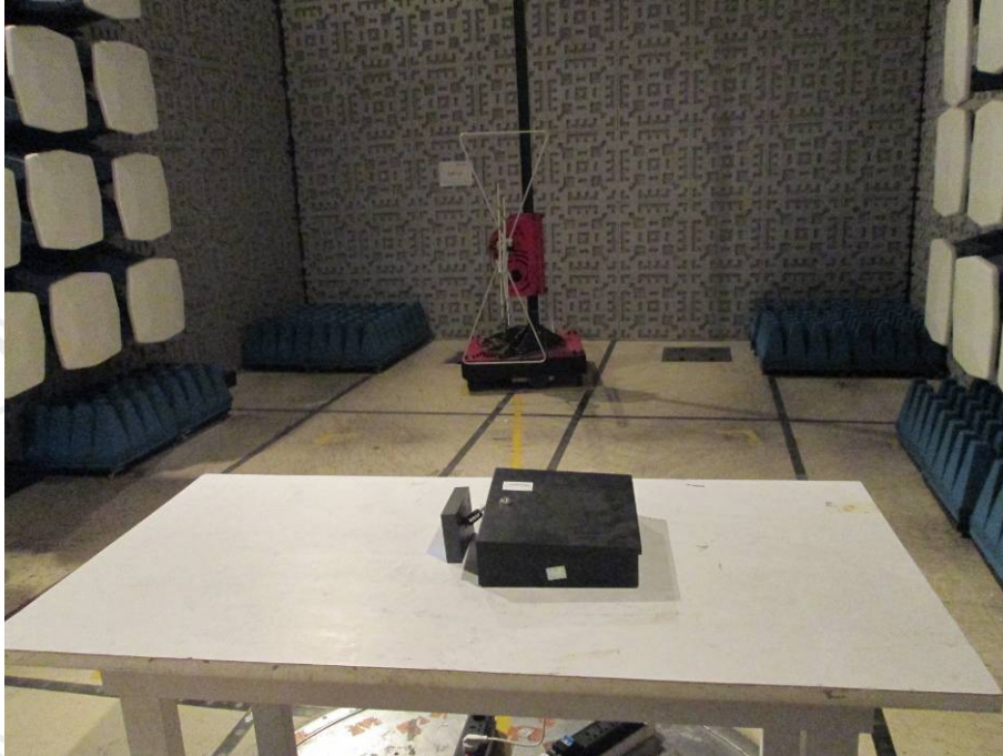
TEST SETUP OF RADIATED EMISSION (30MHz~1GHz)
