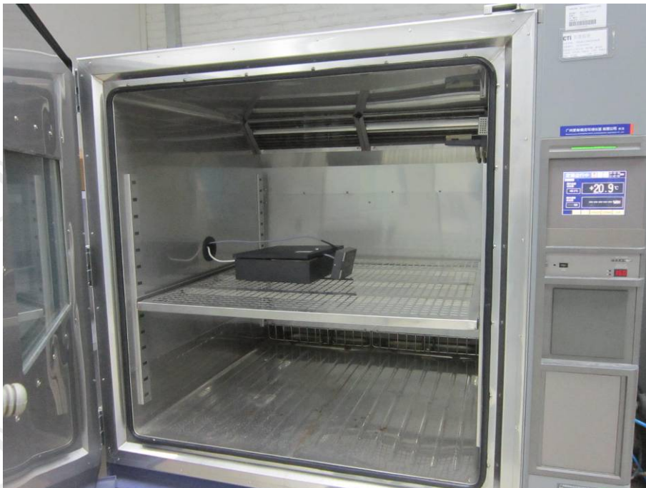
TEST SETUP OF TRANSMITTER FREQUENCY STABILITY
