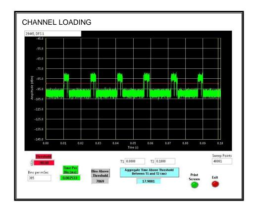
The level of traffic loading on the channel by the EUT is 17.90%.
