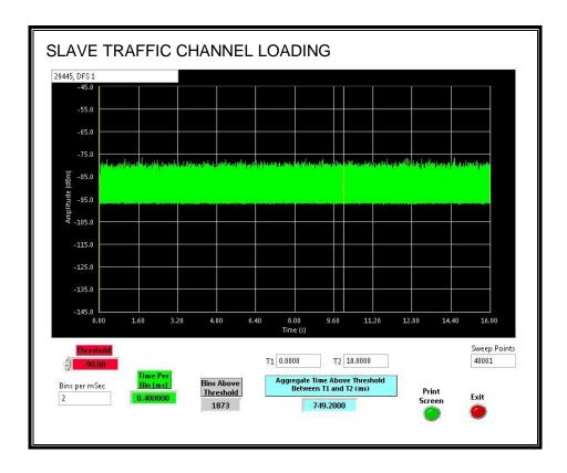
The level of traffic loading on the channel by the EUT is 7.49%.
