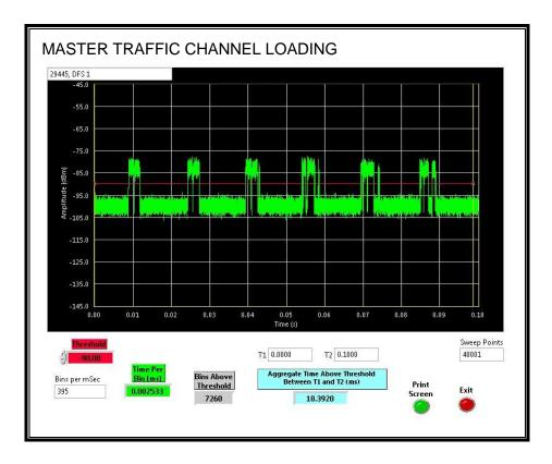
The level of traffic loading on the channel by the EUT is 18.39%.
