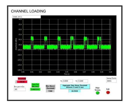
The level of traffic loading on the channel by the EUT is 18.39%.
