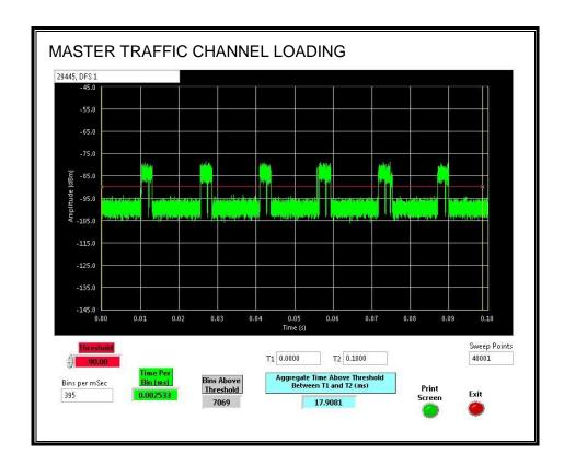
The level of traffic loading on the channel by the EUT is 17.9%.
