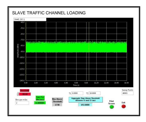
The level of traffic loading on the channel by the EUT is 6.92%.
