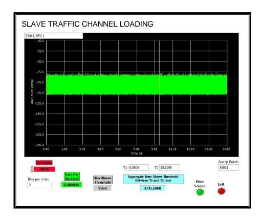
The level of traffic loading on the channel by the EUT is 37.45%.
