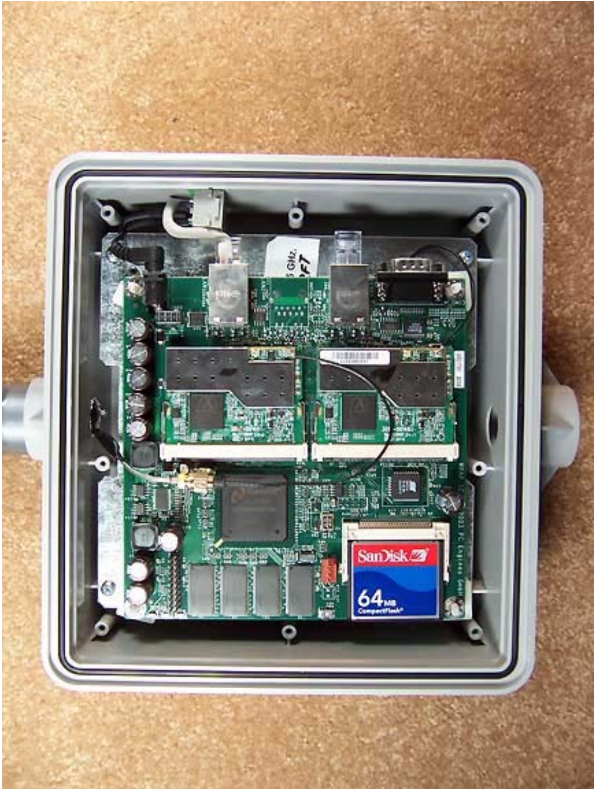
Relay Internal PCEngines
