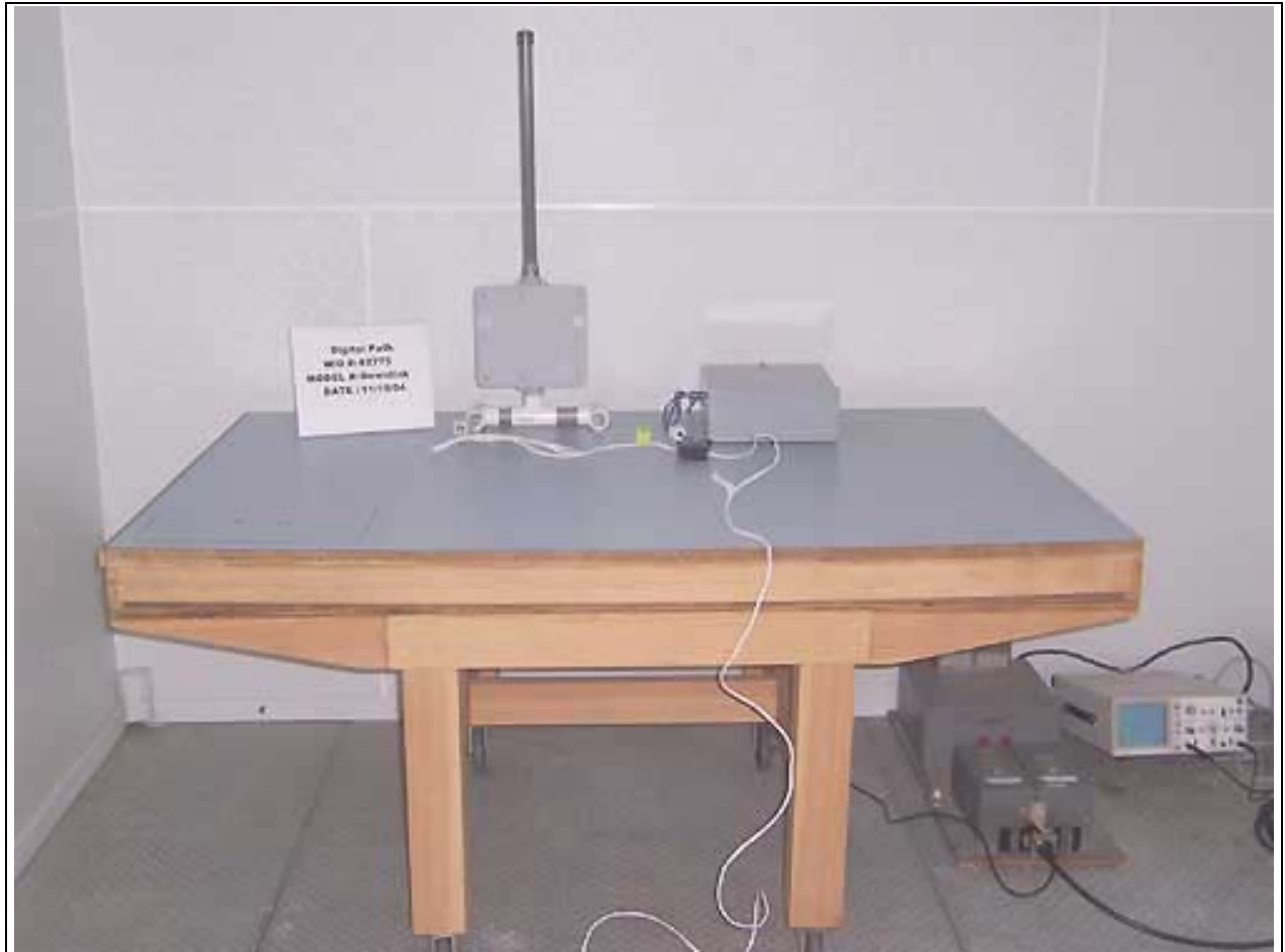
Mains Conducted Emissions - Front View
