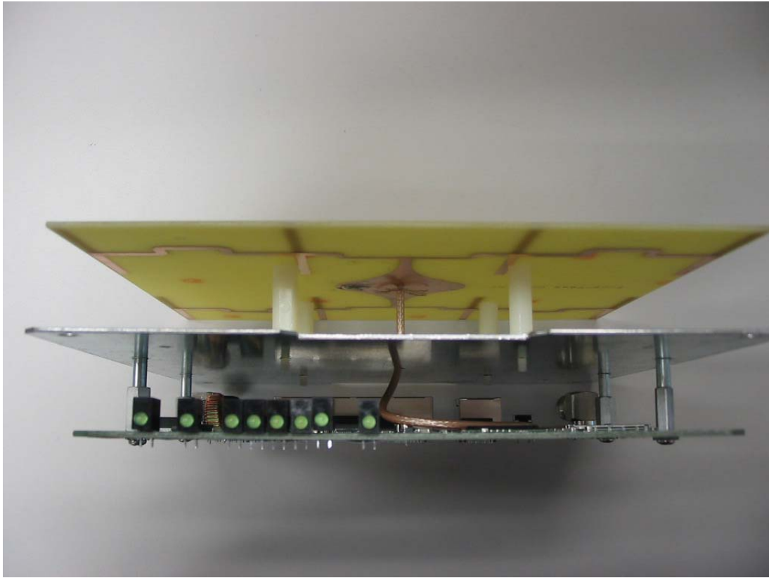
Assembled PCB w/ direct solder to Antenna Top View
