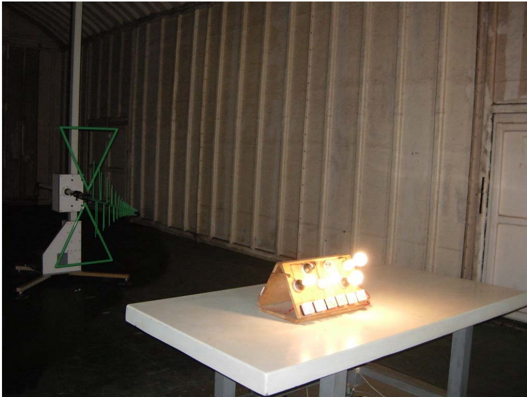
Back View of Radiated Test
