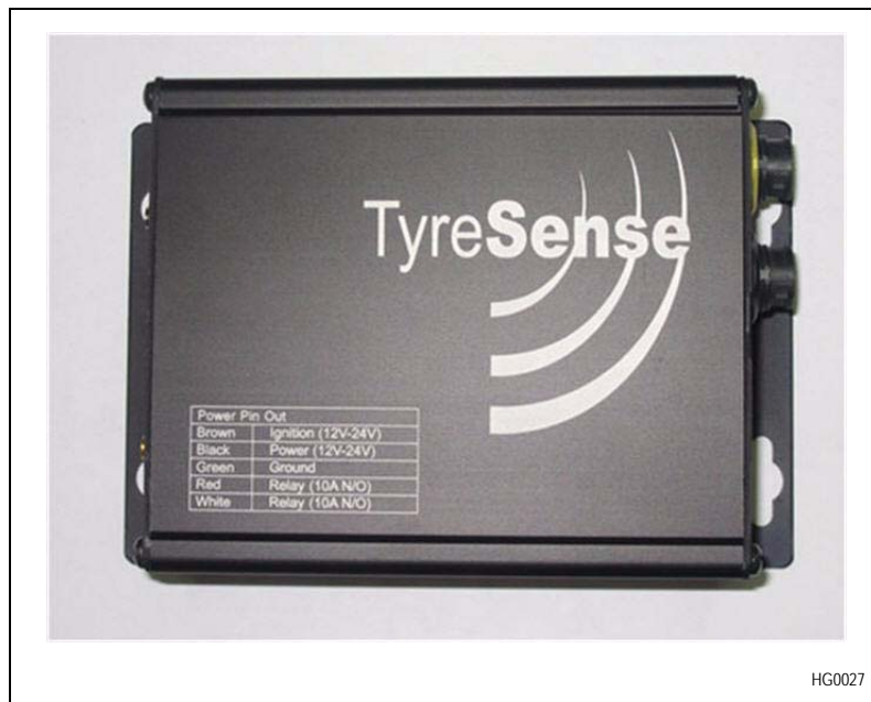
Figure 4-1 – Gen II Receiver Unit top plate
