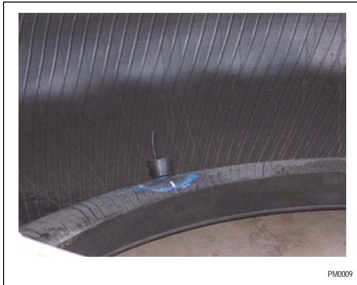
Figure 16-6 – Installed patch mount wheel sensor
