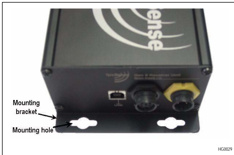
Figure 4-3 – Gen II Receiver Unit mounting brackets and holes
