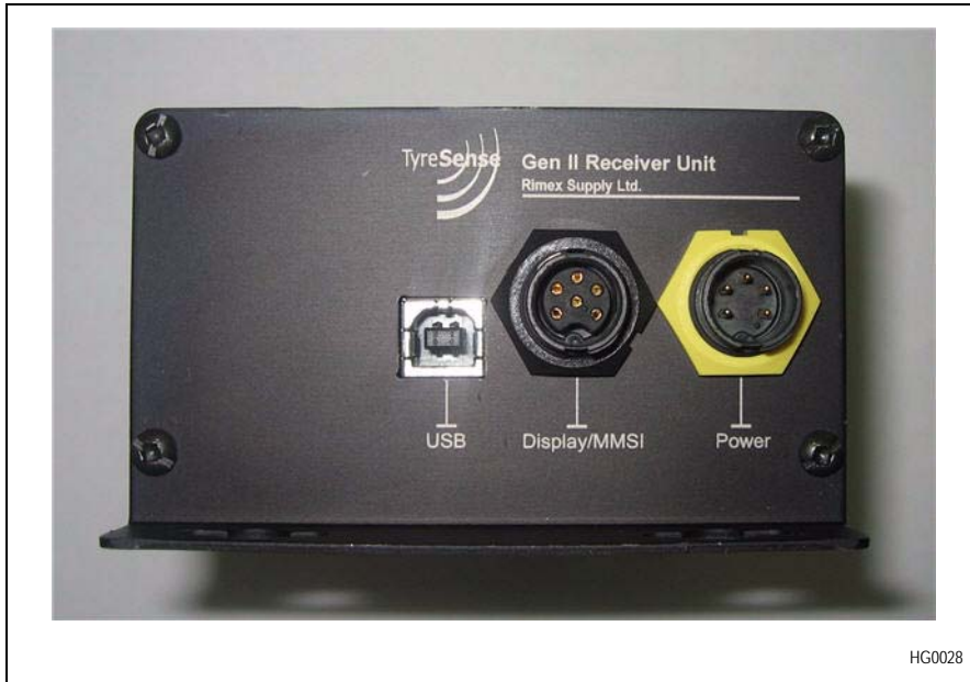
Figure 4-2 – Gen II Receiver Unit power endplate
