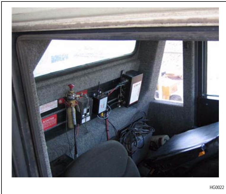
Figure 4-4 – Example of Gen II Receiver Unit mounting location
