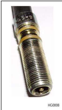
Figure 17-3 – O-rings on the PT valve
