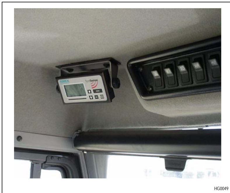
Figure 3-3 – Gen II Display Unit mounted on the ceiling of the cabin
