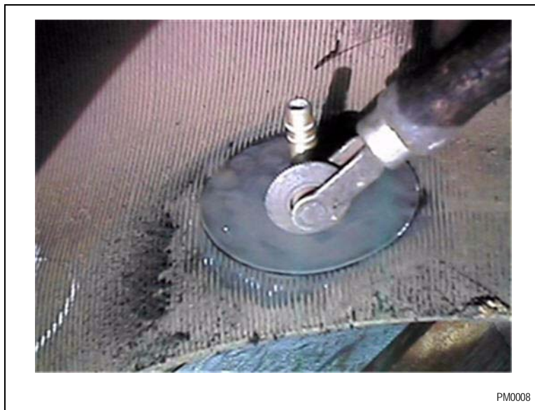
Figure 16-5 – Stitching the patch mount
