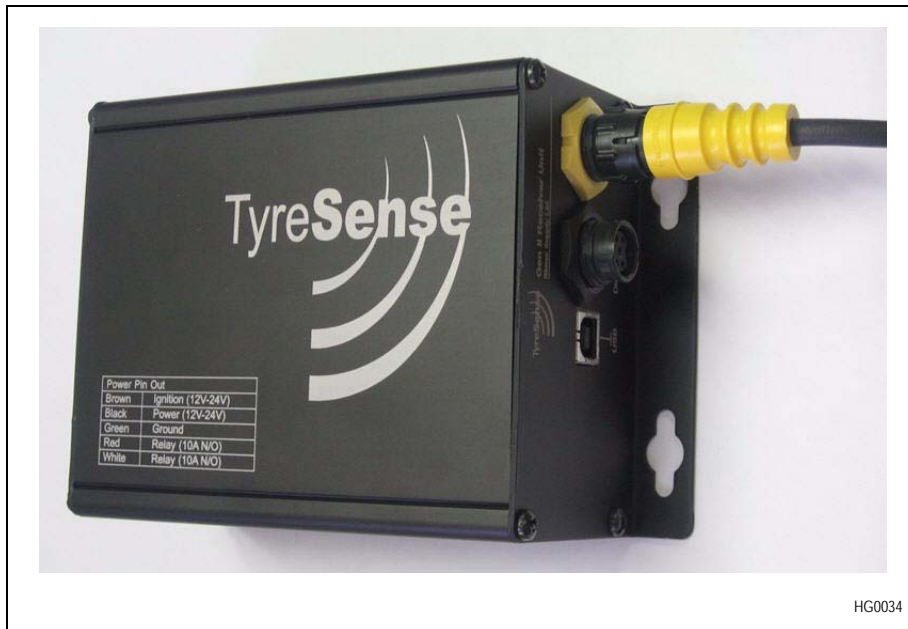
Figure 5-2 – Installed power cable
