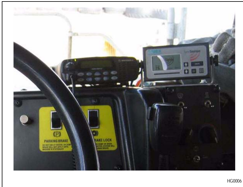
Figure 3-2 – Gen II Display Unit mounted on the dashboard of a vehicle
