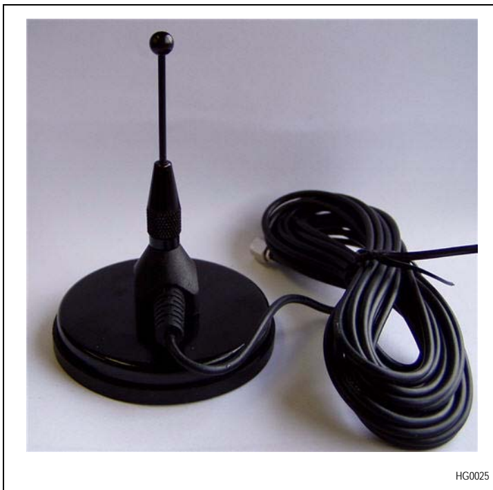
Figure 10-5 – Assembled base mount antenna
