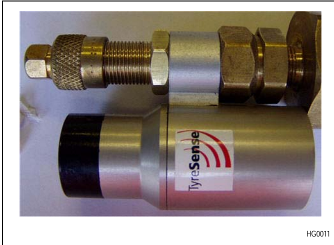
Figure 17-7 – Valve mount sensor installed on PT-EX adapter
