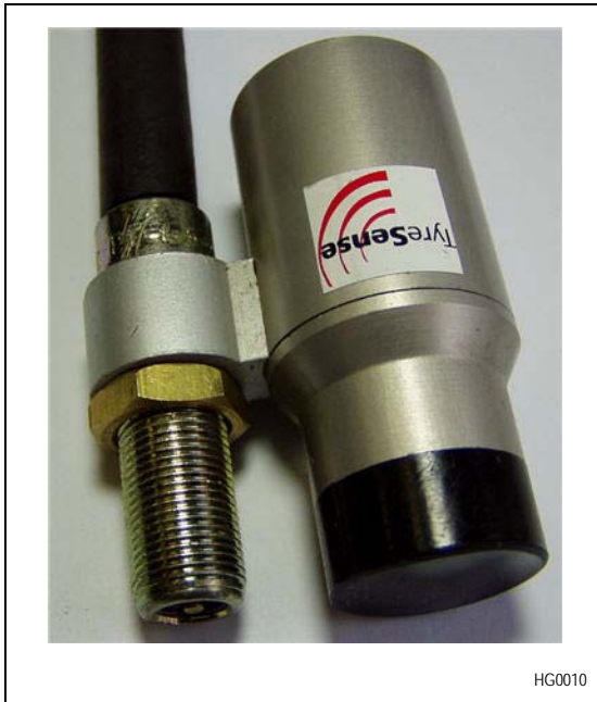
Figure 17-5 – Valve mount sensor and brass retaining nut
