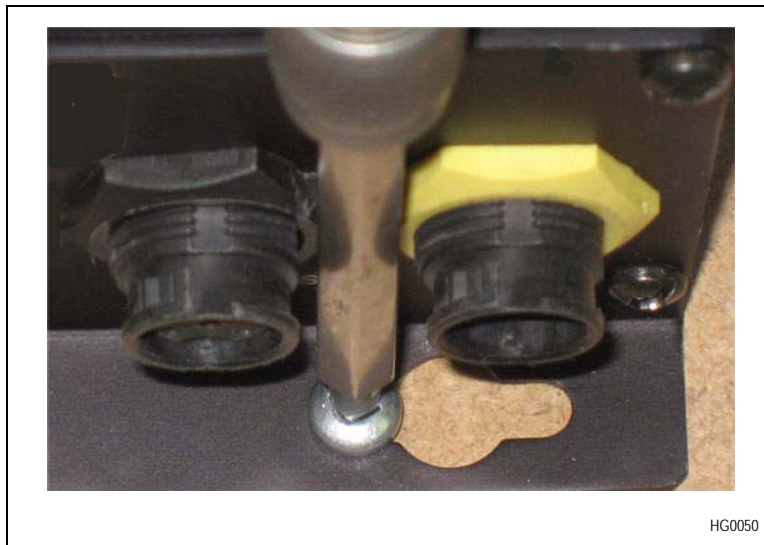
Figure 4-5 – Mounting the Gen II Receiver Unit
