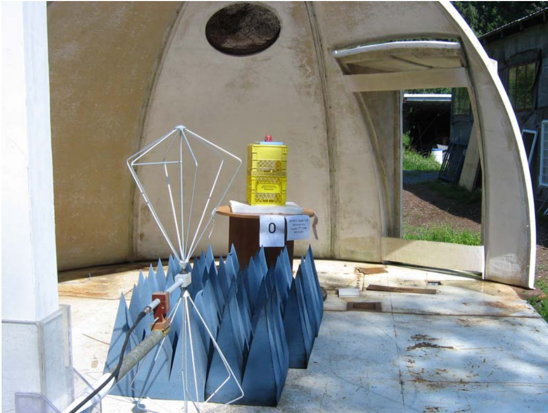
Pic 1: Emissions Test Set-up of EUT during Radiated Emissions Testing
