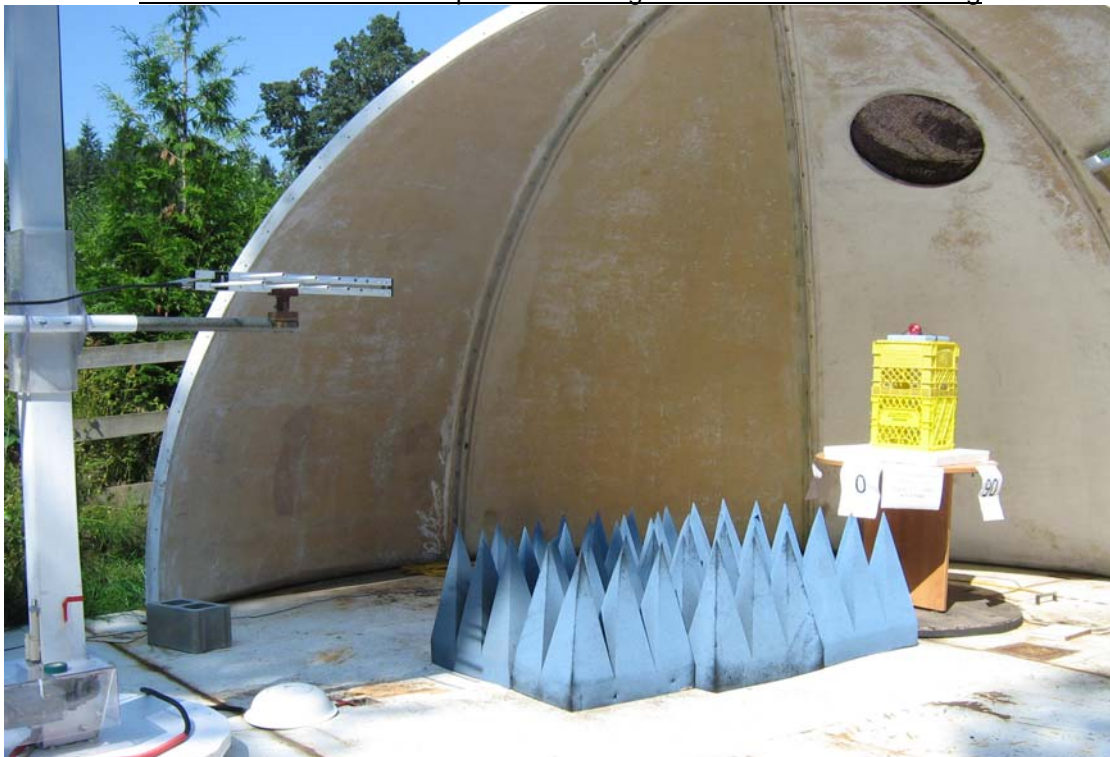
Pic 4: Emissions Test Set-up of EUT during Radiated Emissions Testing
