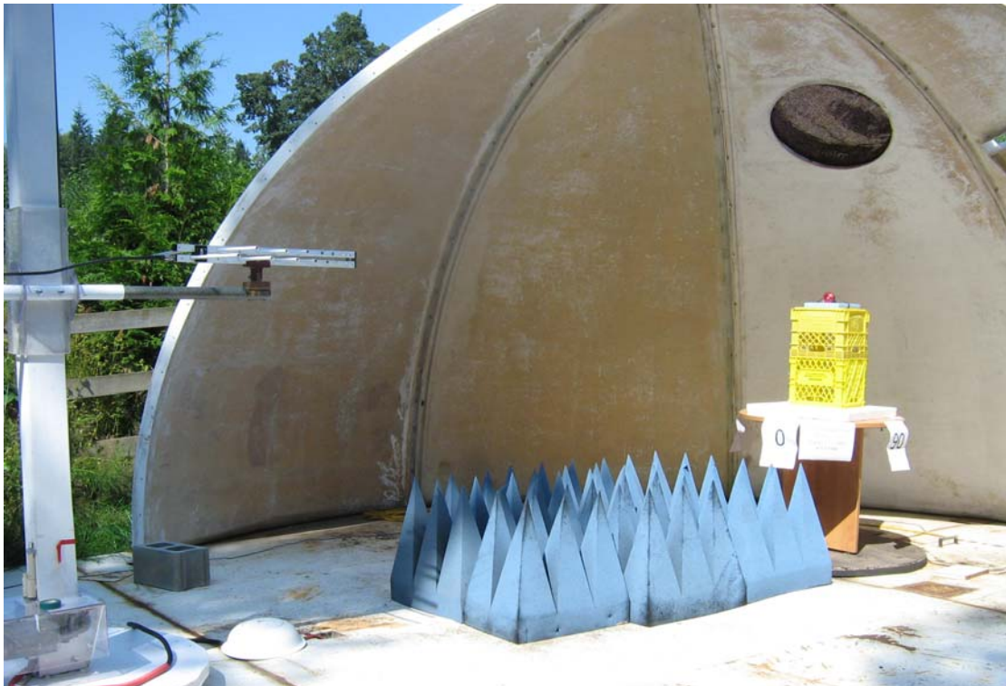
Pic 3: Emissions Test Setup of EUT during Radiated Emissions Testing
