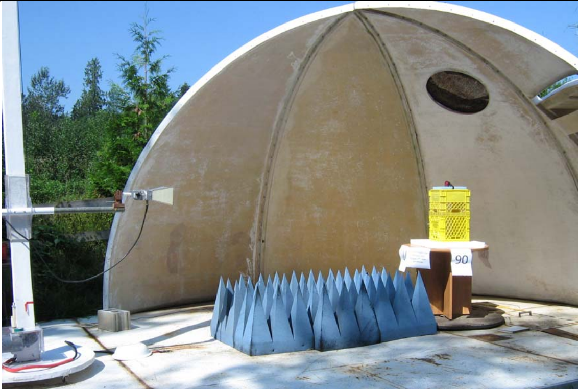
Pic 3: Emissions Test Setup of EUT during Radiated Emissions Testing
