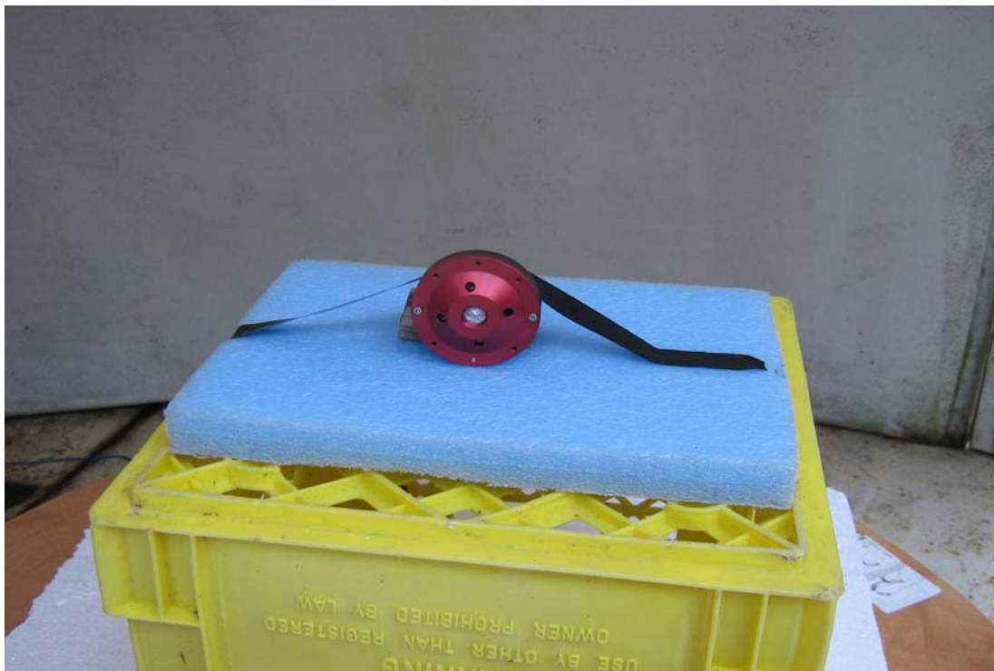
Pic 2: Emissions Test Set-up of EUT during Radiated Emissions Testing
