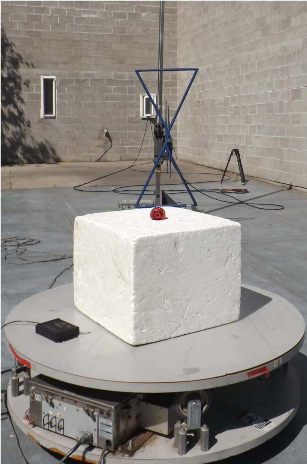
Figure E21.4 – Setup Photo – Radiated Emissions, 30 – 1000MHz, Vertical
