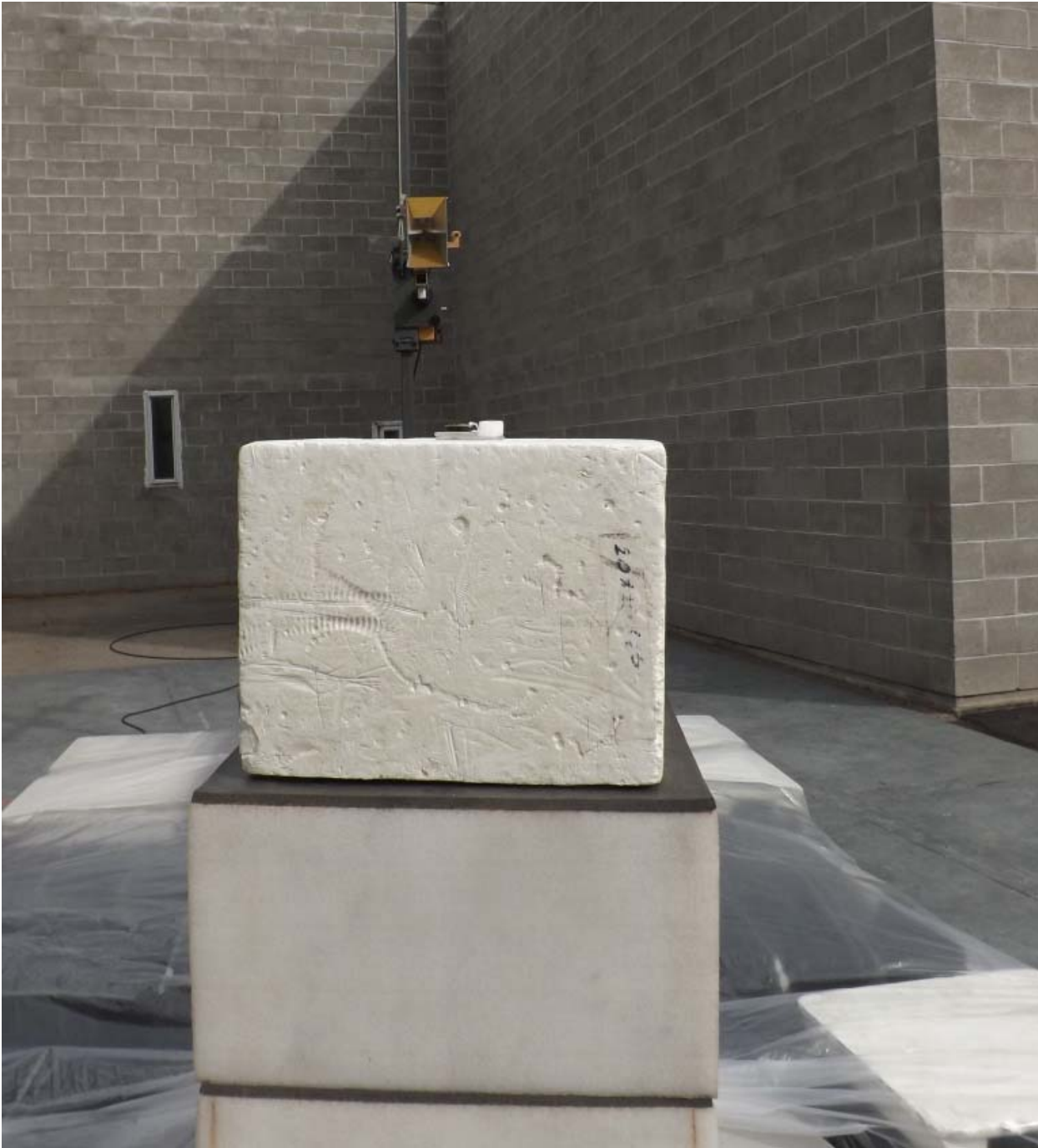
Figure E21.5 – Setup Photo – Radiated Emissions, 1 – 18GHz, Horizontal
