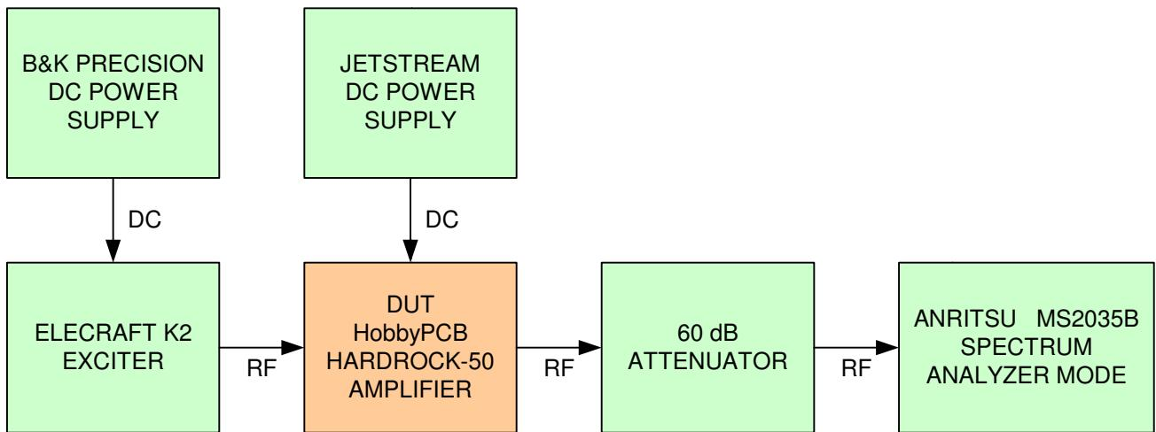
Gain measurements are made with the following procedure:
