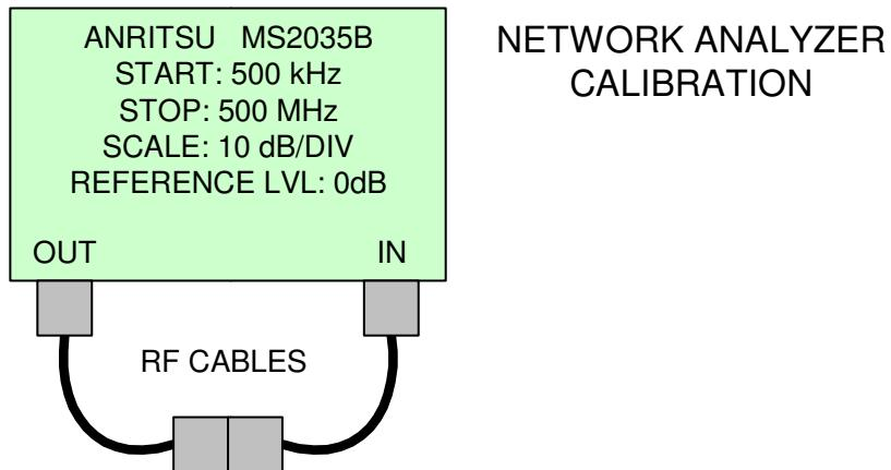
The NA is then calibrated using the internal calibration routine and the attenuator is inserted at the reference plane:
