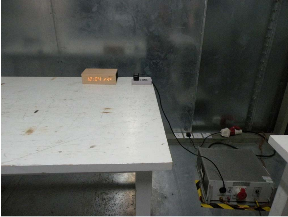
Radiated Emission Test Setup in Chamber
