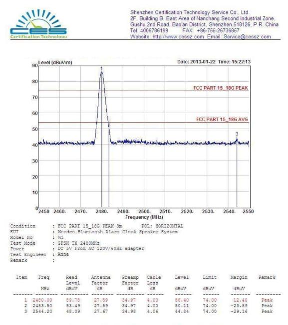
Remark: Level = Read Level + Antenna Factor - Preamp Factor + Cable Loss
