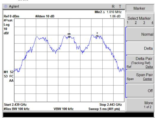
Orginal test data for channel separation GFSK
