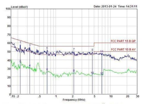
POL: LINE Temp:24 C Condition : FCC PARI 15 B QP Hum:56 % : Wooden Bluetooth Alarm Clock Speaker System EUT Model No : W1 Test Mode : Working Power : DC 5V From AC 120V/60Hz adapter Test Engineer: Eric Remark :
