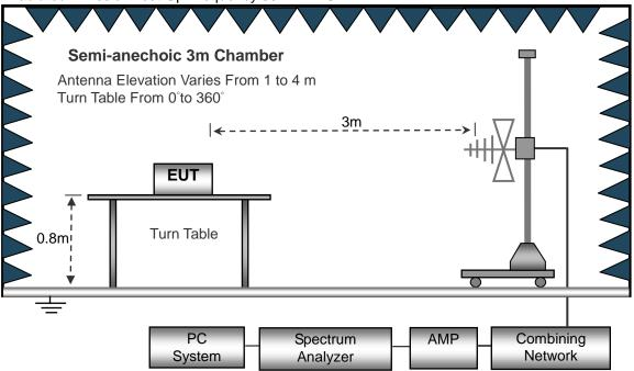
(C) Radiated Emission Test-Up Frequency Above 1GHz
