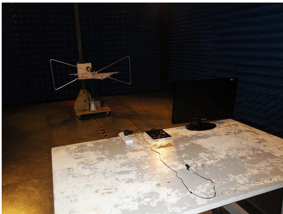
Radiated Emission Test Setup:
