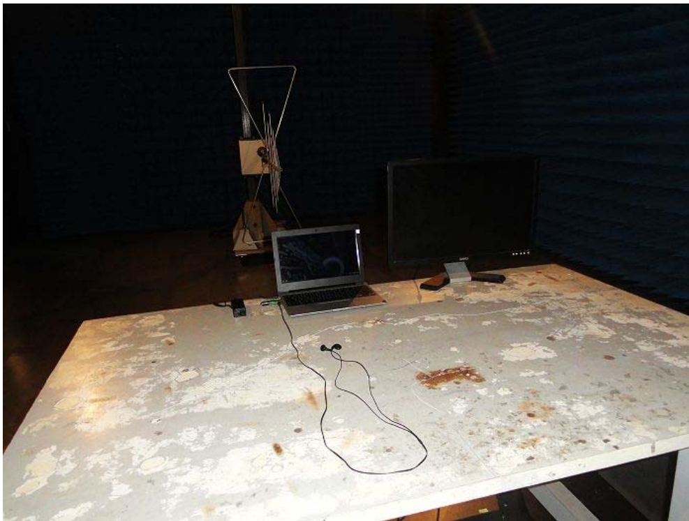
Radiated emission test view--
