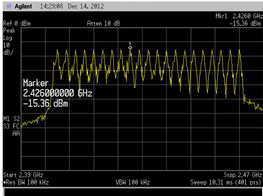
The channels were observed between 2402 MHz and 2462 MHz with 3 MHz channel spacing
