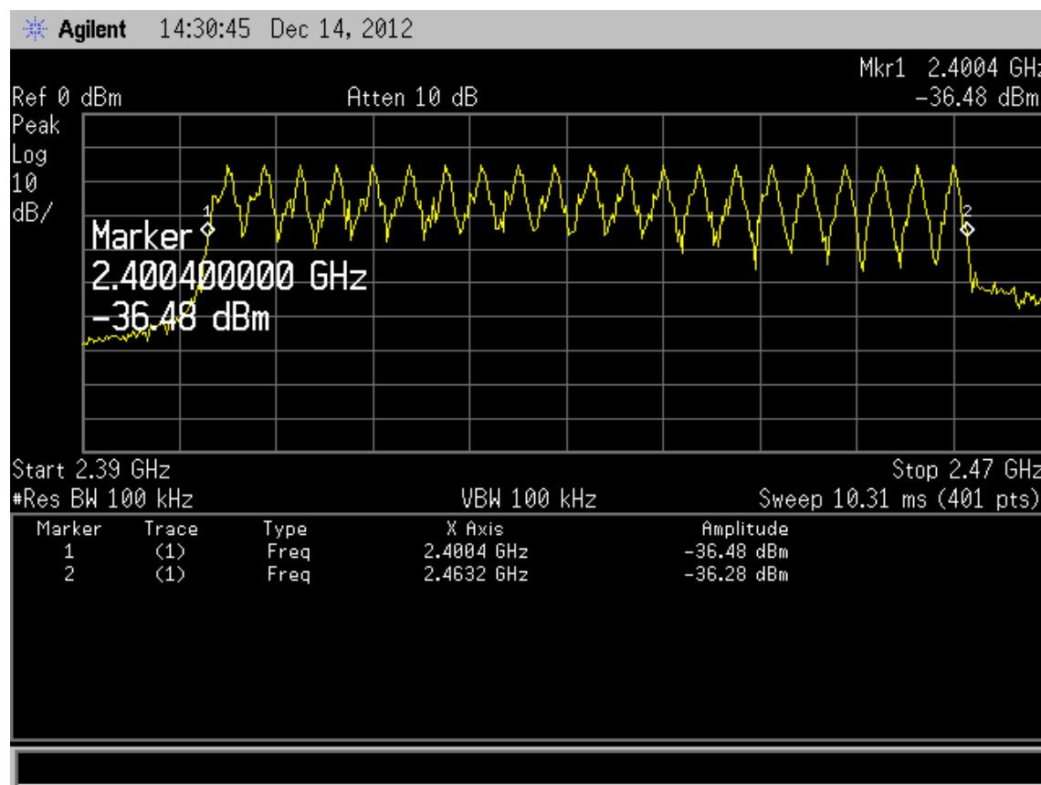
In addition radiated measurements were made in the restricted bands of 2310 – 2390 MHz and between 2483.5 – 2500 MHz where the limits as defined in section 15.209 were applied.
