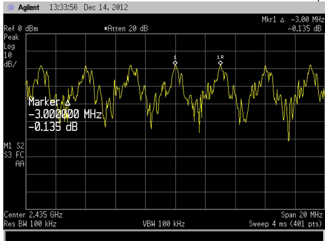
The -20 dB bandwidth for each device has been determined below
