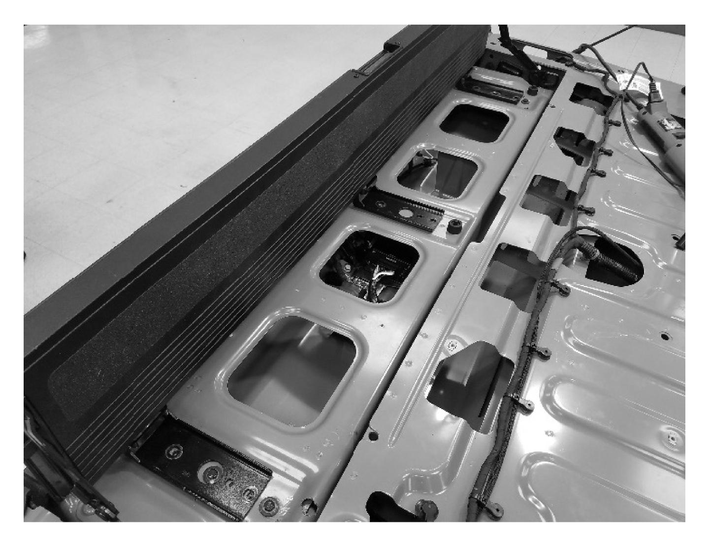
21. Vacuum any metal shavings created during the drilling process from inside the tailgate
