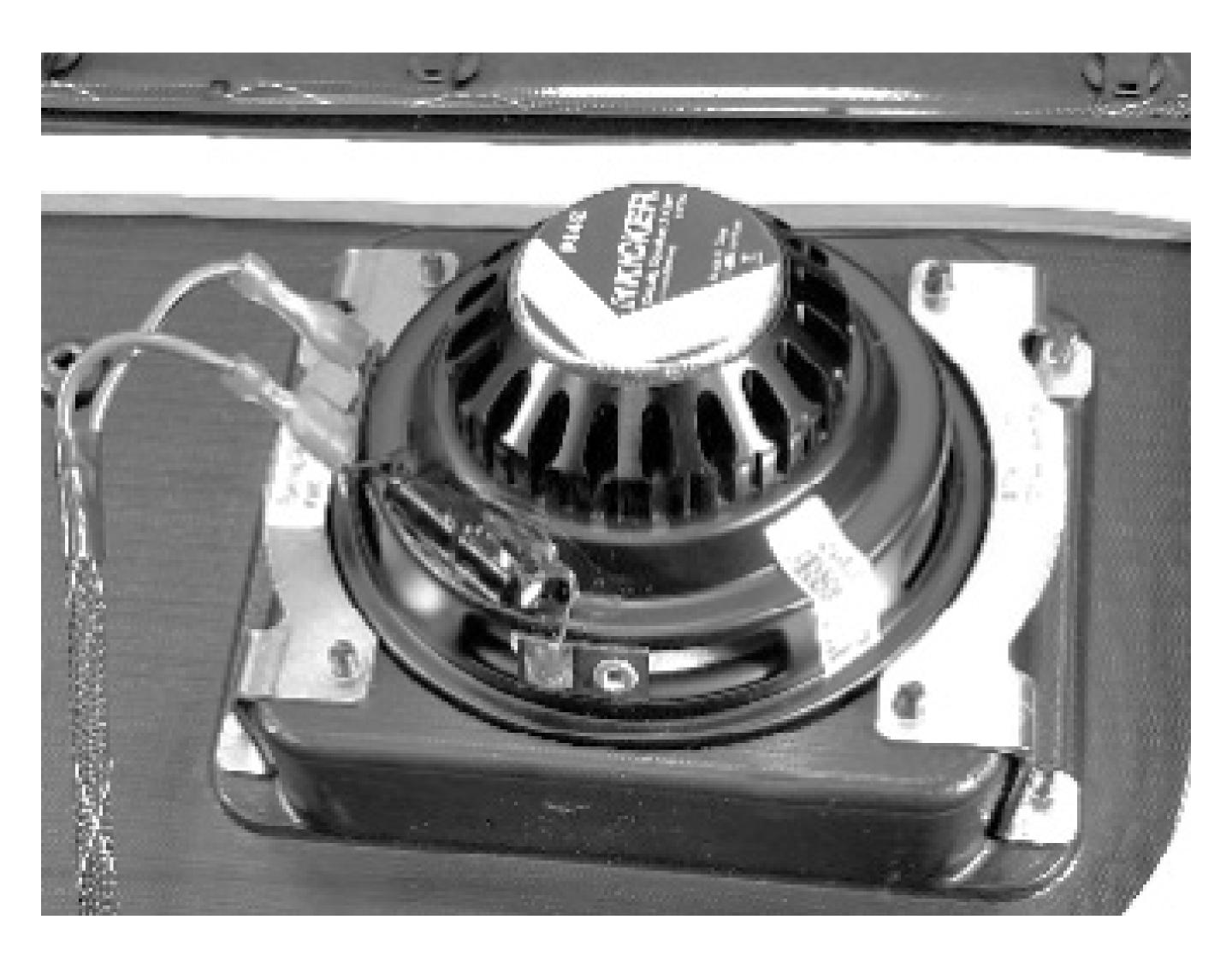
27. Secure extra controller cable with wire ties.
