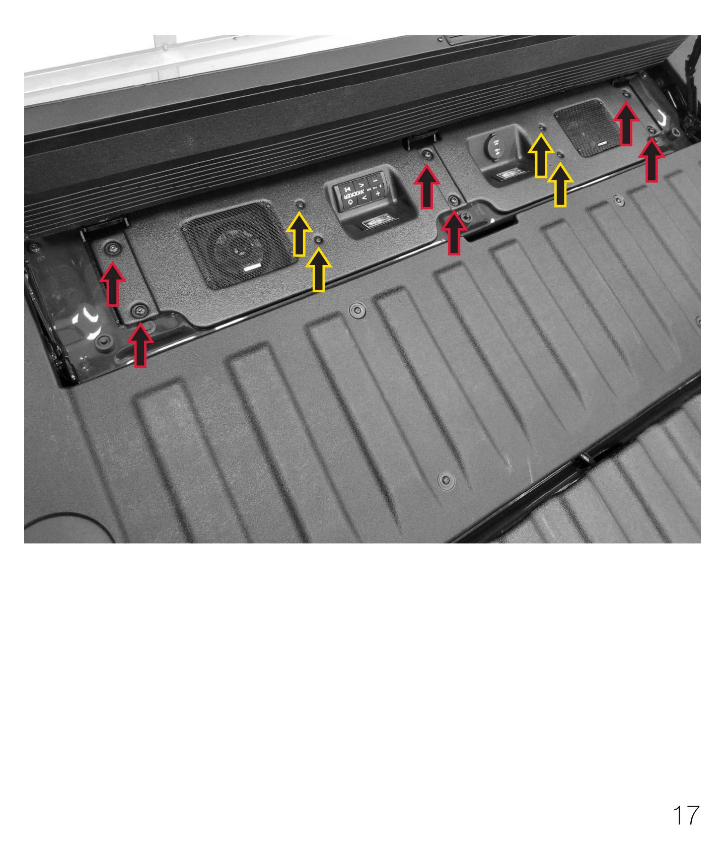
33. Close the step over the speaker baffle and check clearance from step to baffle. If additional clearance is needed open inner tailgate and loosen the two hinge bolts on each side. Slide step away from baffle and retighten hinge bolts. Recheck clearance and make sure step still closes easily.
