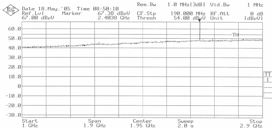
Note: The peak above the limit is the carrier frequency.
