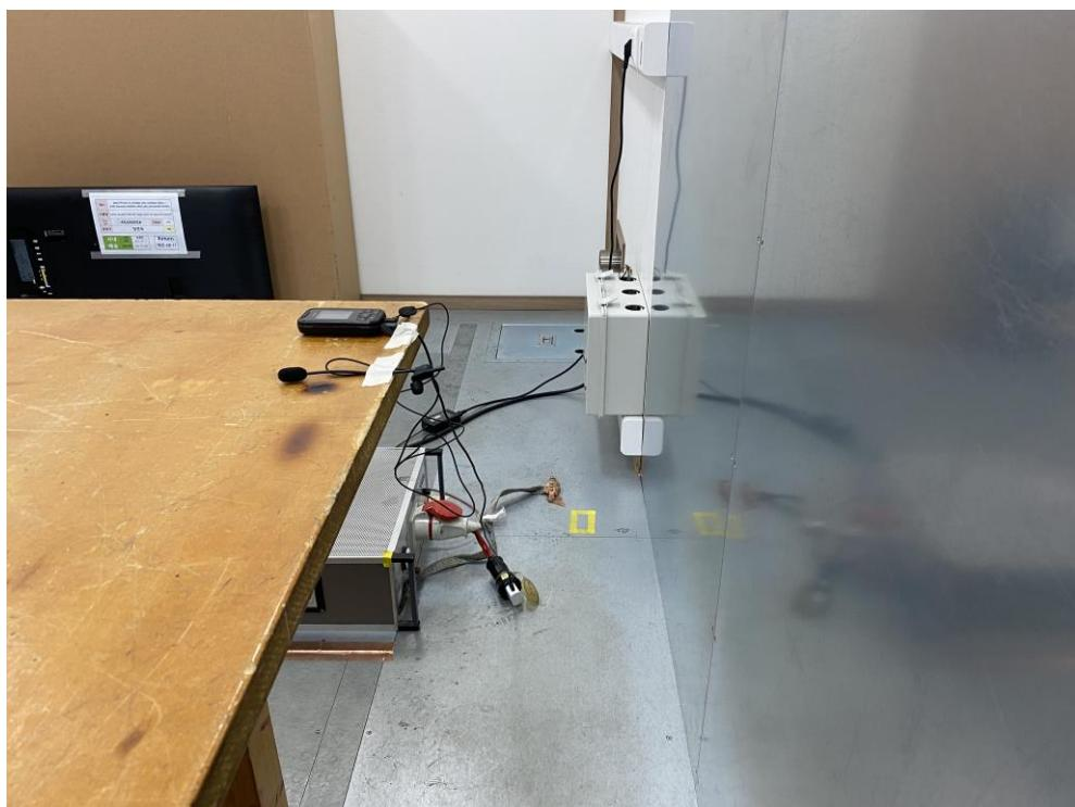
**- Radiated Emission Test (Below 30 MHz)**
