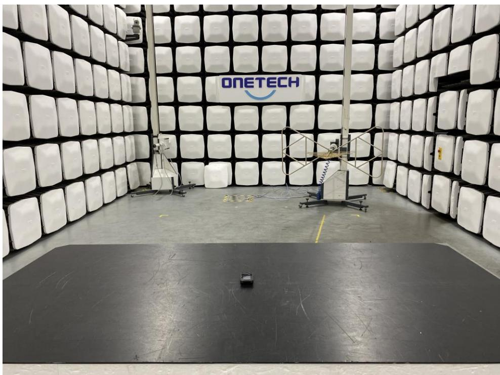
**- Radiated Emission Test (Above 1 GHz)**
