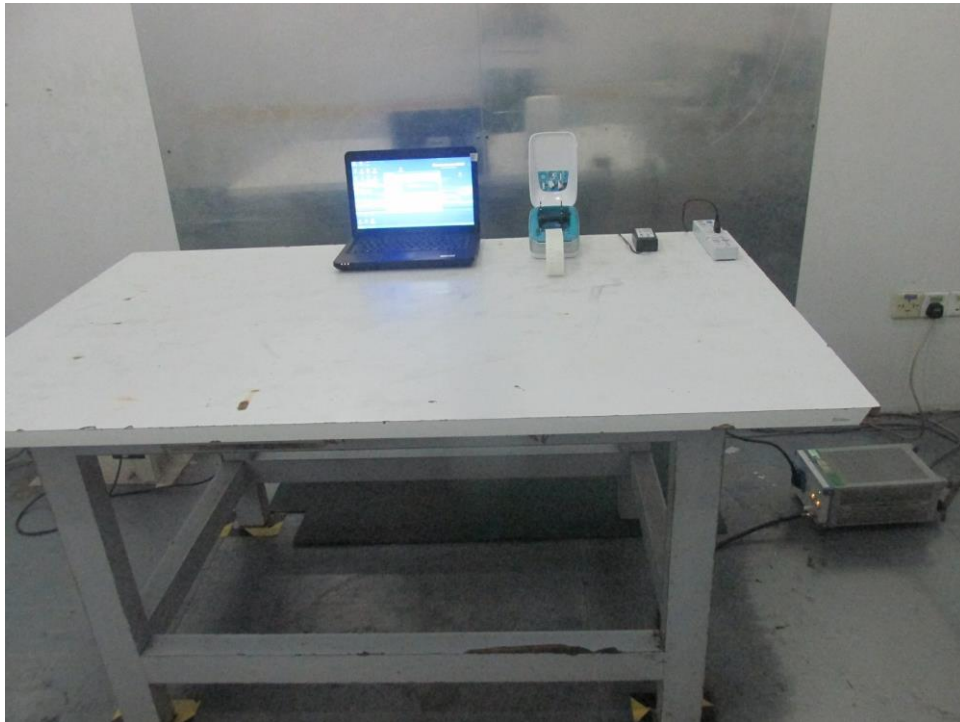
Photograph 5: Setup for Conducted emissions on AC Mains
