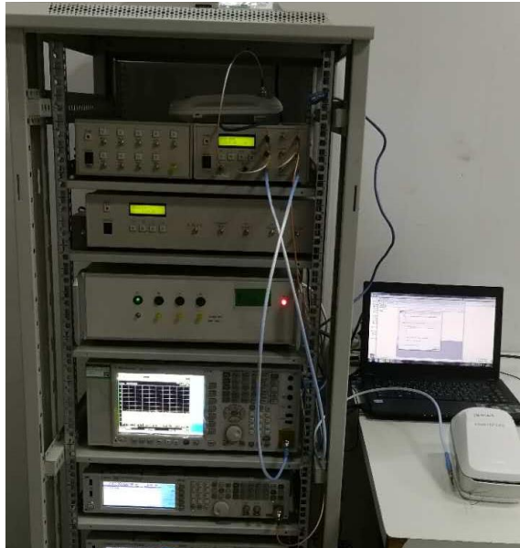
Photograph 2: Setup for Spurious emissions, 30MHz-1GHz
