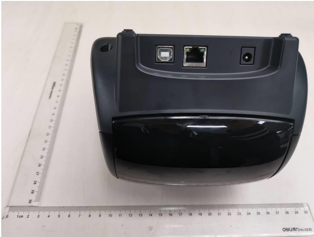
Fig 5: Rear view (DC jack, RJ45 connector and USB connector view)
