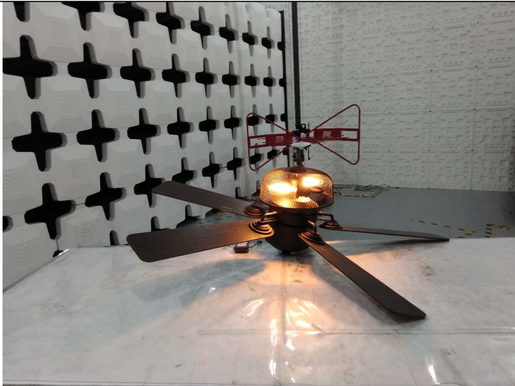
Radiated emission Test Setup-1 (30 MHz~1 GHz)
