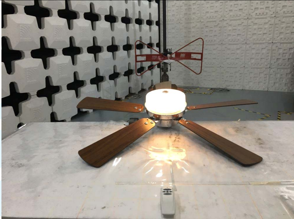
Radiated emission Test Setup-1 (30 MHz~1 GHz) - Mode 1
