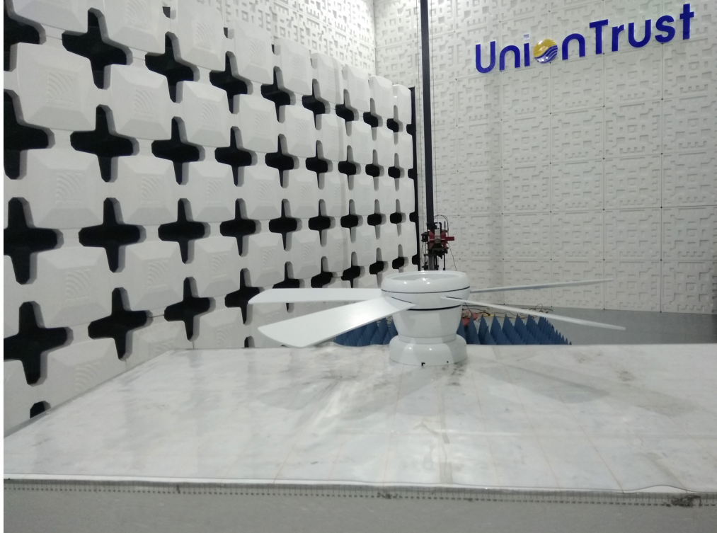
Radiated emission Test Setup-2 (Above 1 GHz) - Mode 1
