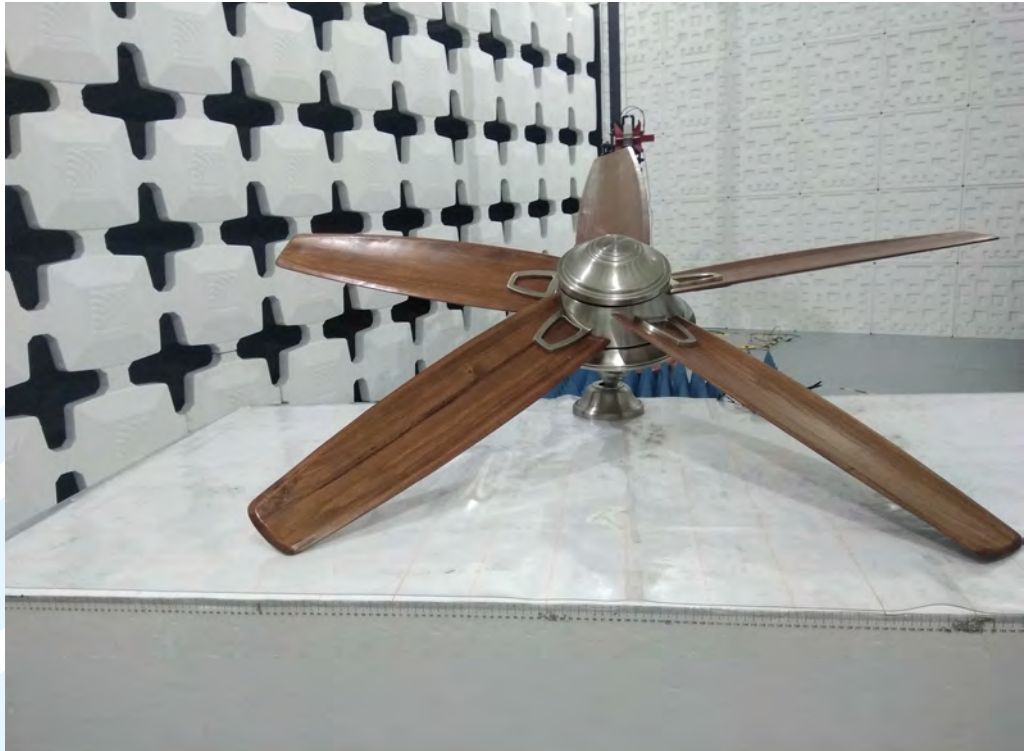
Radiated emission Test Setup-2 (Above 1 GHz) - Mode 1
