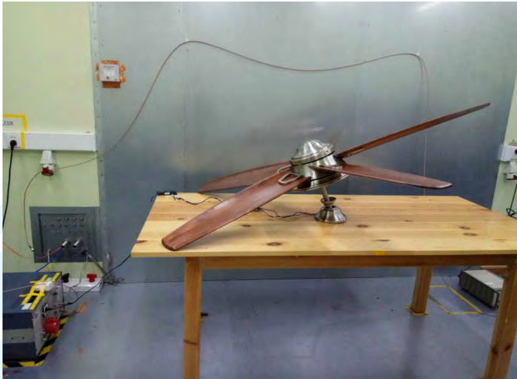
Conducted Emission Test Setup-3 - Mode 1
