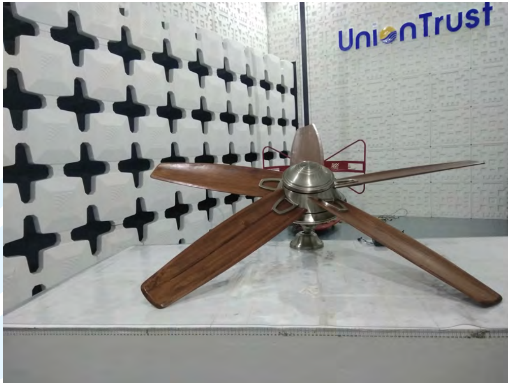
Radiated emission Test Setup-1 (30 MHz~1 GHz) - Mode 1
