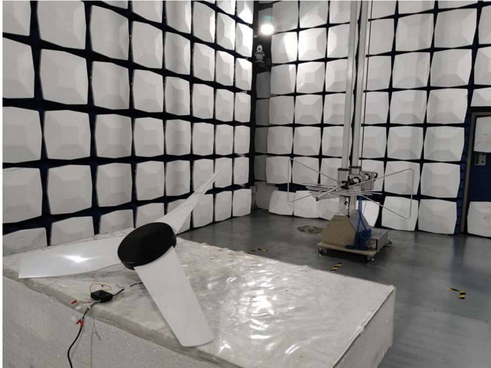
Radiated Emission Test Setup:
