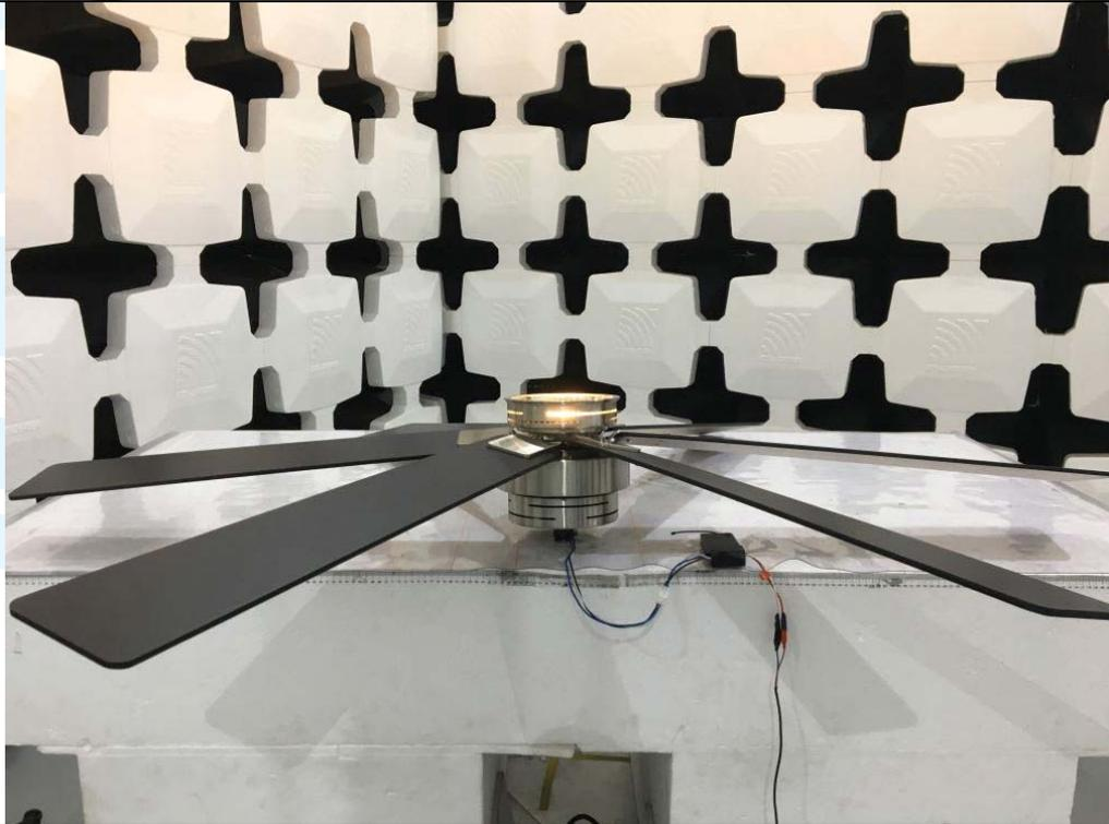
Radiated emission Test Setup-2 (Above 1 GHz) - Mode 1
