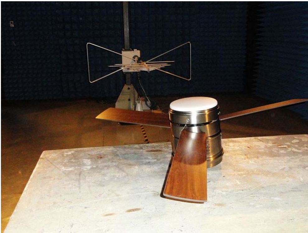
Radiated emission test view--
