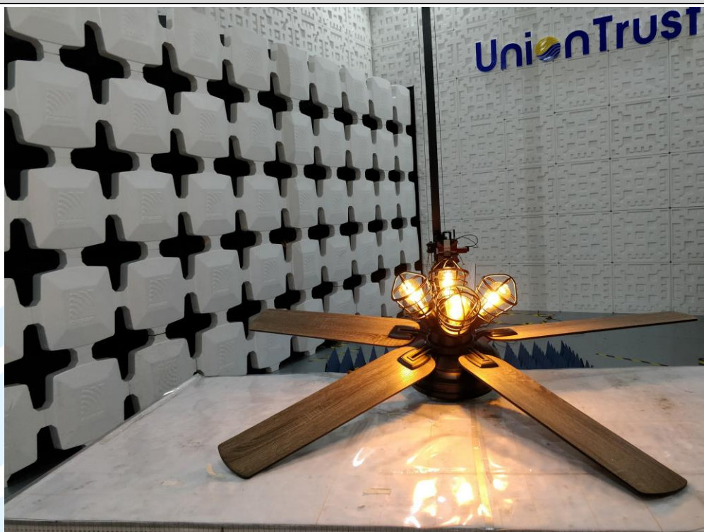
Radiated emission Test Setup-2 (Above 1 GHz)
