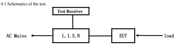
EUT: Equipment Under Test
