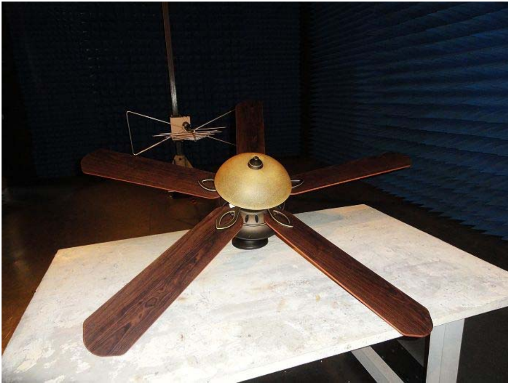
Radiated emission test view--
