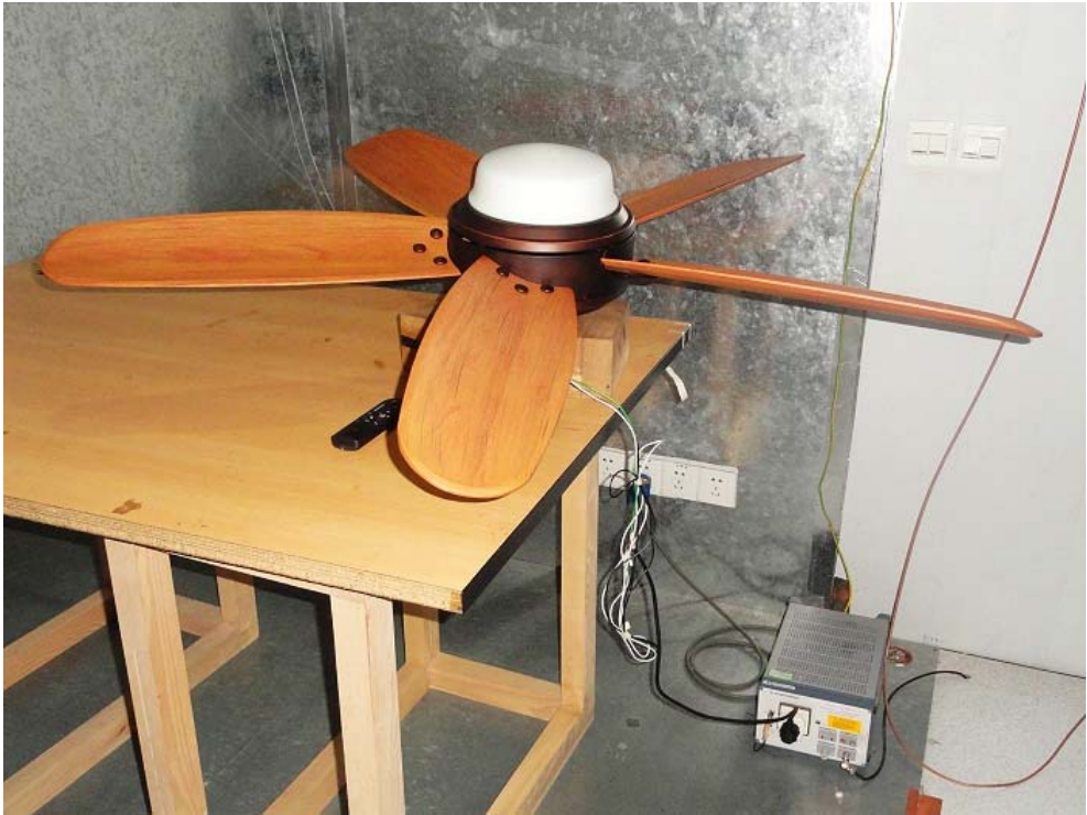
Conducted test View--
