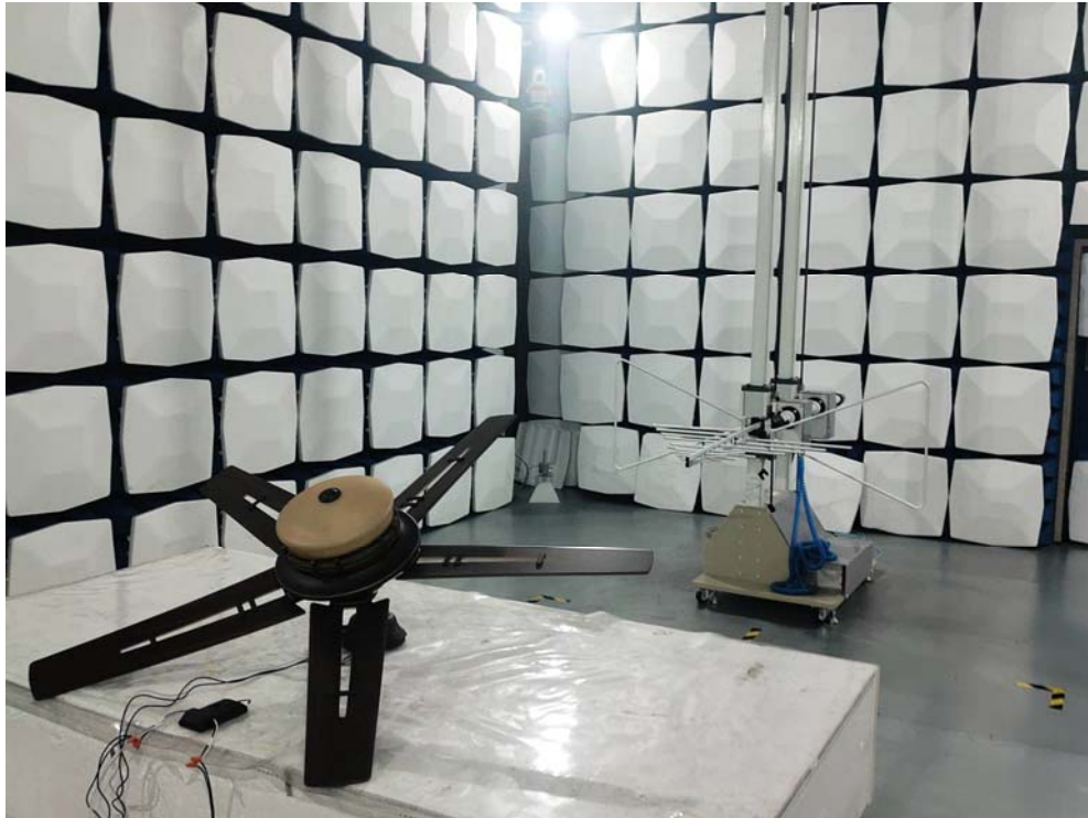
Radiated Emission Test Setup:
