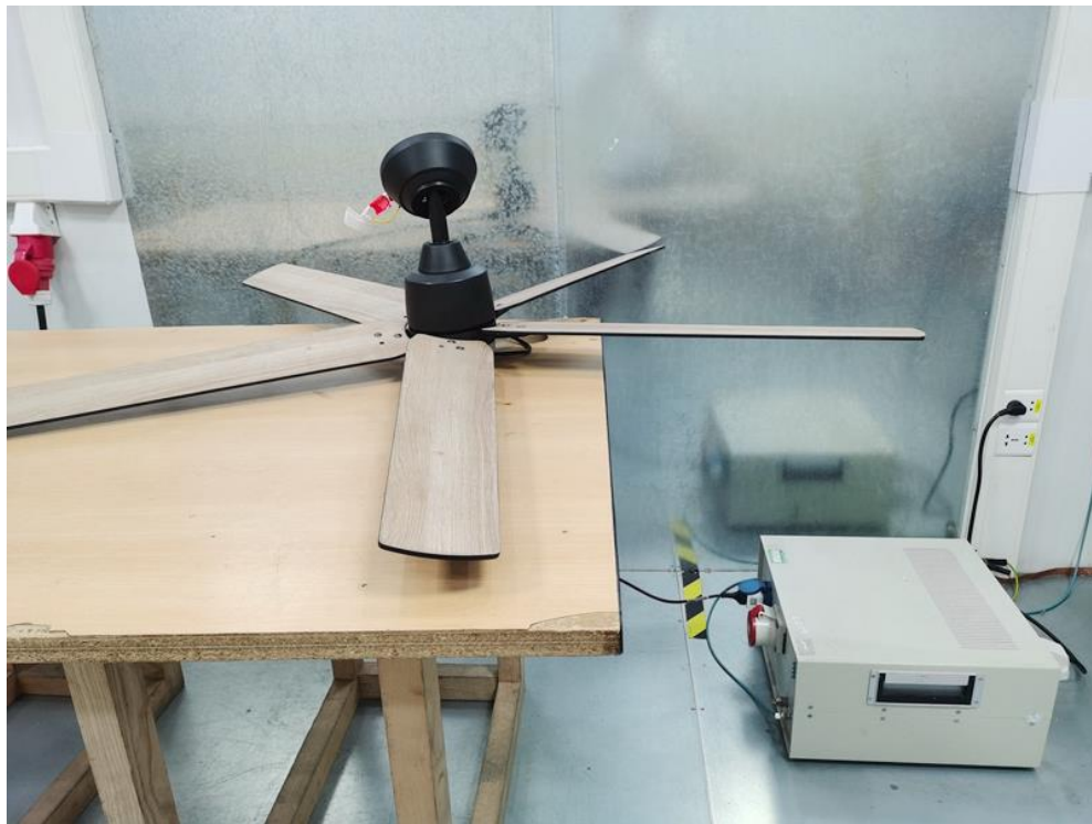
Conducted Emission Test Setup:
