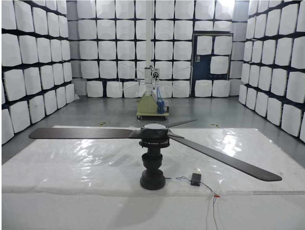
Radiated Emission Test Setup:
