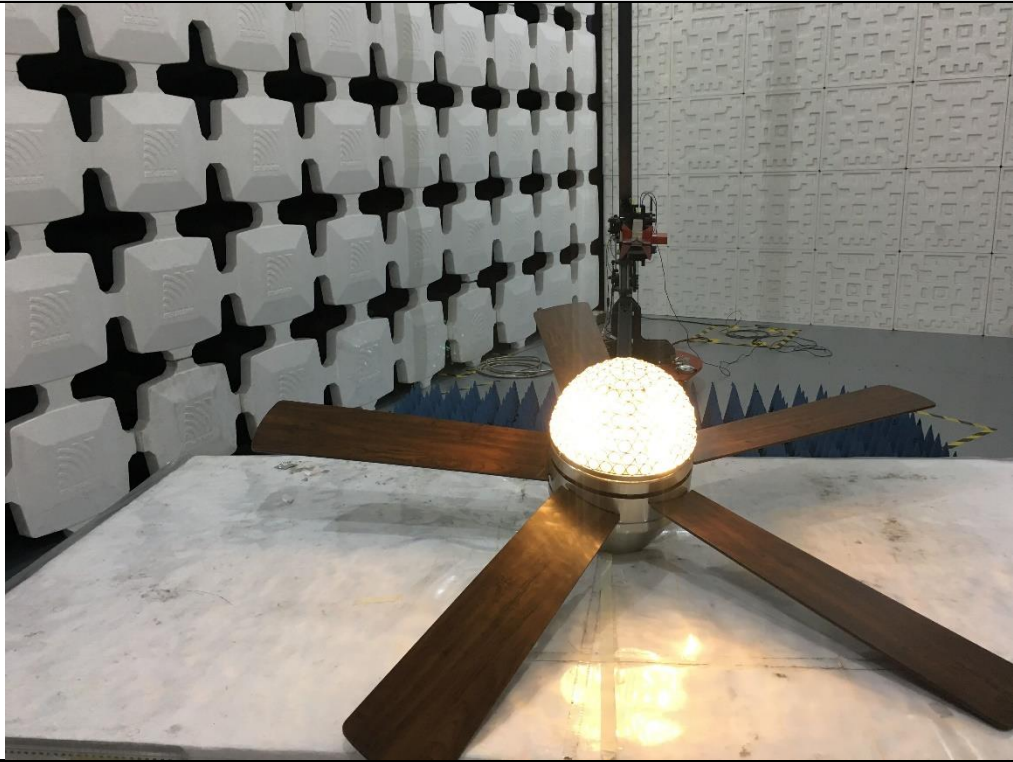
Radiated emission Test Setup (Above 1 GHz)
