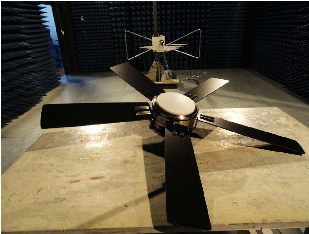
Radiated emission test view--
