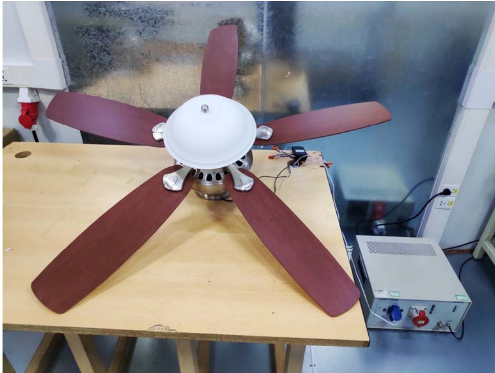
Conducted Emission Test Setup:
