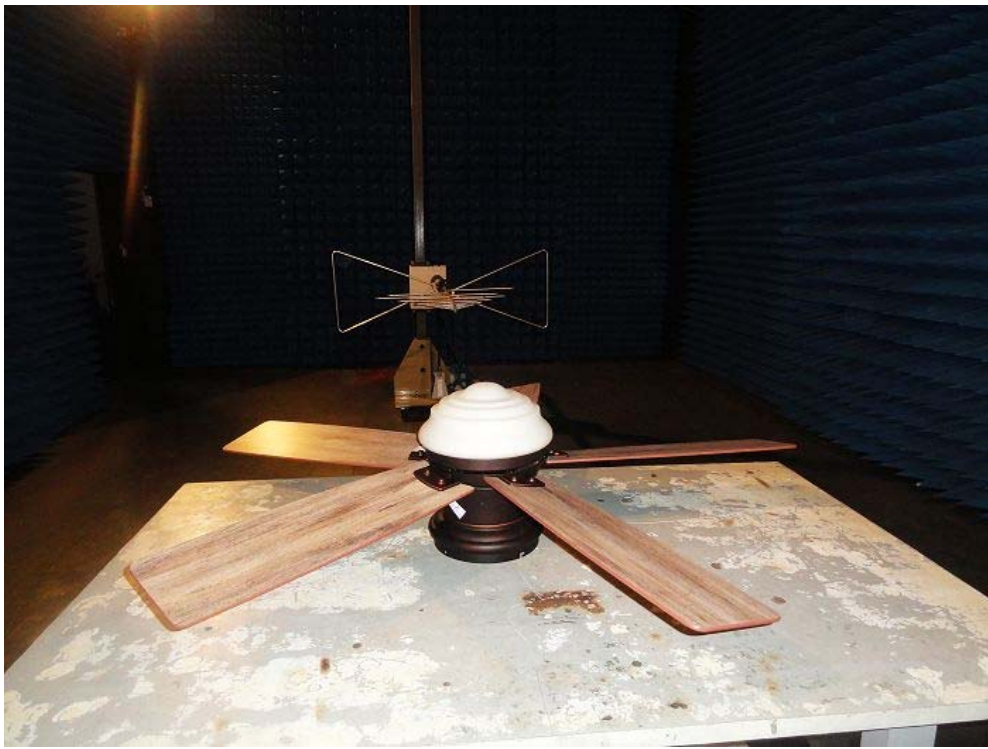
Radiated emission test view--
