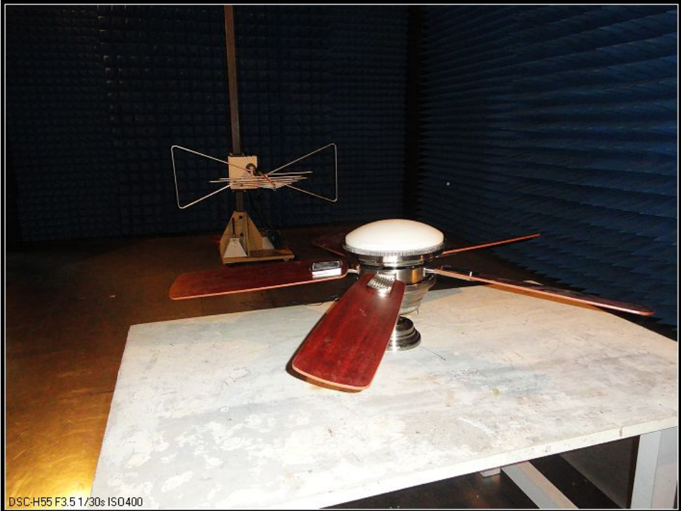
Radiated emission test view--
